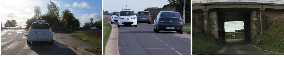
Figure 1: Tornado project key scenarios demonstration. Left graphic corresponds to a roundabout entrance. Centre graphic depicts a narrow two-way road with a gutter. Right graphic plots a non-visibility tunnel crossing with a reduction from two-way to a single lane.
