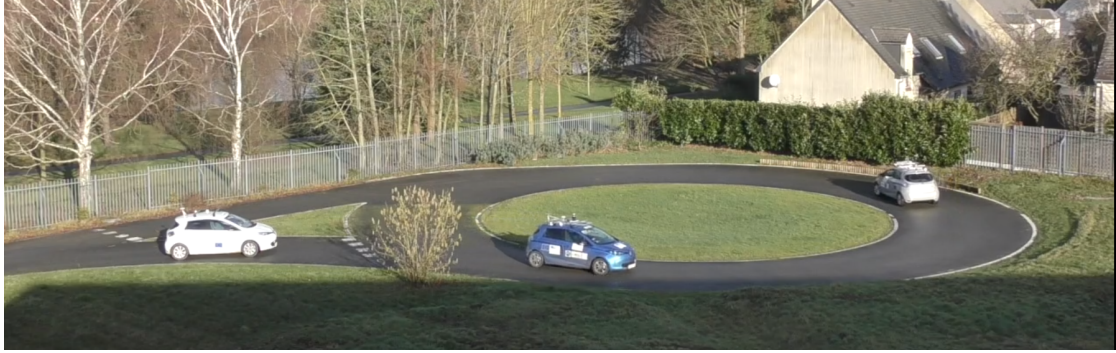
Figure 52: The experimental circuit “Seville” and the experimental Renault Zoé’s used during the real outdoor tests. In our configuration, the white car (fully autonomous) is the AD vehicle, while the others are the road users (manually driven).
